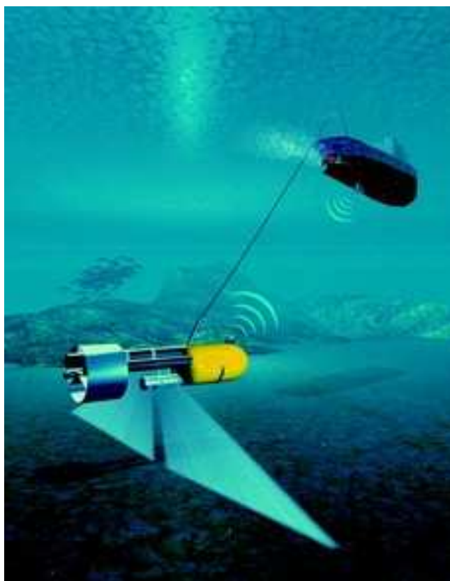
Figure 19 GAPS fixed on the hull and a transponder on a tow fish
