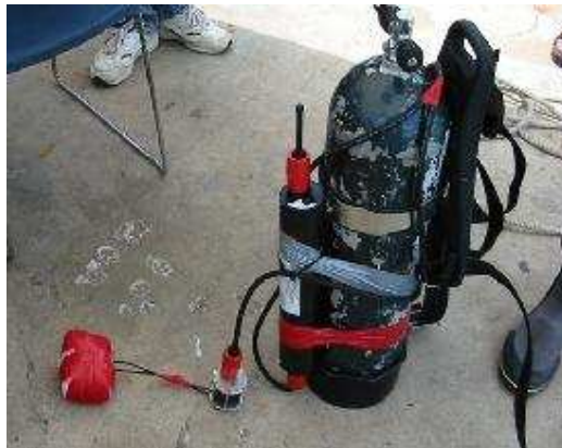
Figure 21 - Transponder fixed on a scuba cylinder
