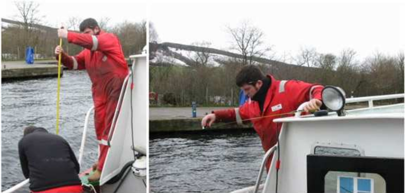
Figure 32 – Measure of GPS lever arms with respect to GAPS
