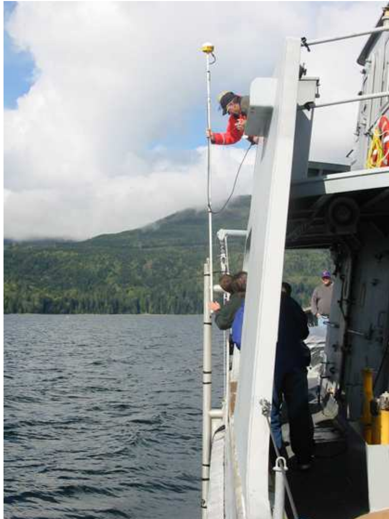
Figure 27 - DGPS antenna installation
