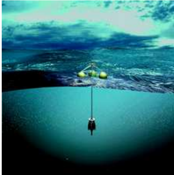
Figure 20 - GAPS mounted under a tripod
